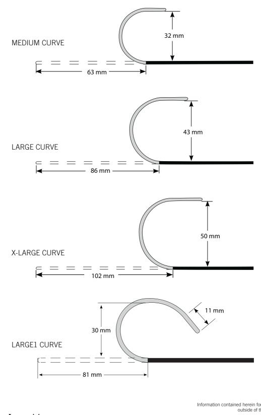
Safire<sup>™</sup> BLU<sup>™</sup> Duo and Therapy<sup>™</sup> Cool Path<sup>™</sup> Duo Ablation Catheters (Bi-directional) 4 mm Tip Curve Reference
