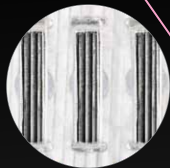
Close-up of electrodes with micro-texturing
