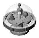
Geometric Phantoms provide a full independent check that head rings, localizers, CT or MRI scan images, and planning software all deliver accurate volumetric target localization.
